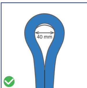
Minimal diameter of bending is 40mm. Excessive bending may result in damaging the source of light.
