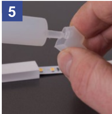
5 Carefully slide the LED strip back into the silicone encapsulation. Fill the end cap up to ¾ of its volume with neutral silicone.
