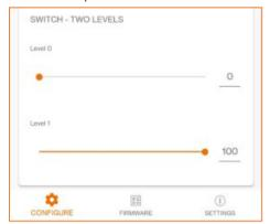
When the switch is closed (short circuit) the output will go to Level O.
