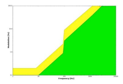
Thanks to its 3,4kHz dimming frequency, the LINE-4CC-CASAMBI effectively reduces the occurrence of the Flicker phenomenon. Depending on an individual's sensitivity and the nature of their activities, flickering can impact one's well-being, even if the changes in luminance are beyond the threshold detectable by the human eye.
