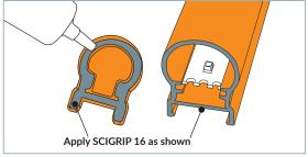
**4.** Apply a generous, continuous bead of SCIGRIP 16 to both the end-cap and the cut end of the Hi-Lite™ 30 section. Do not substitute any alternative adhesive or sealant. Use **SCIGRIP 16** in a well ventilated area, following the safety instructions on the tube.
