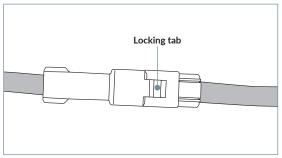
10. In order to maintain weather sealing connections must be properly made. When connected correctly the two halves will be locked together and will not pull apart without first releasing the locking tab.
