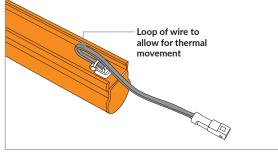
**5.** If a standard section is to connect to further sections loop the output connection as shown before fitting the tube into position. Leave a loop of cable to allow for movement due to thermal expansion and contraction.
