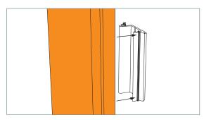
**4.** On vertical installations, the high-friction clip is particularly important to prevent Hi-Lite™ 30 sections from slipping down over time.
