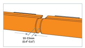
**12. DO NOT** butt sections up together. Doing so will cause the sections to bend in warm weather. Leave 10-15mm (0.4"-0.6") gap for thermal expansion. In very cold weather a larger gap may be required. If the Hi-Lite™ 30 sections are installed at a 2.4m (7'10½") pitch, the required expansion gaps will automatically be present.
