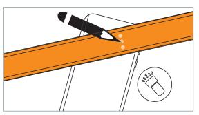
**1.** Field Adjustable Hi-Lite<sup>™</sup> 30 tubes can be cut at specific locations approximately every 50mm (2"). To locate a cut position shine a torch (or smart phone with torch function) from the face side. Cut positions will be seen as a row of three bright dots along the rear of the tube. Mark the required cut position.
