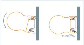
7. Hook the Hi-Lite™ 30 tube section into the top of the clip as shown, then rotate down until the bottom edge clips into place. Ensure the tube is properly located in the clip and that no wires are trapped. A 'click' should be heard when the tube is located correctly.
