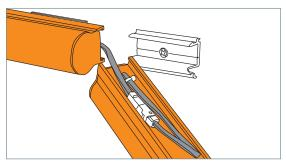
9. Connect the next tube, looping the cable around in the rear channel. Once again leave a loop of cable to allow for thermal movement.
