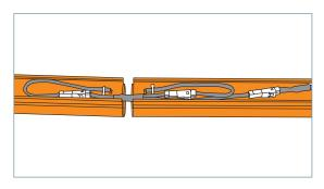
14. 'Y' splitter adapters can be used with Field Adjustable Sections to enable the electrical circuit to continue (around corners for example). The 'Y' adapter can be hidden behind the tube in the same way as a standard connection.
