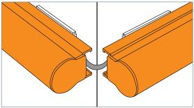
**13.** Hi-Lite<sup>™</sup> 30 tube sections can be run up to the edge of external corners. It is not recommended to overlap the sections.
