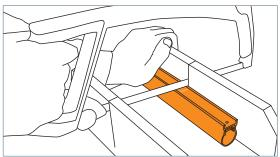
2. Field Adjustable sections must be cut from the connector end only. The portion cut off without a connector is scrap and cannot be used. Cut through the Hi-Lite™ 30 section at your mark using a hacksaw fitted with a fine-toothed blade. Use a mitre box to ensure a clean, square cut.
