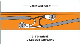
15. If a connection cable needs to be shortened, this can be done using two 3M Scotchlok gel-filled pigtail connectors, such as type UY2. The completed connection can be hidden in the tube channel as shown.
