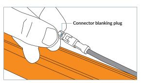
6. If the section is the end of the electrical circuit, a connector blanking plug (supplied with power supply) MUST be fitted to the unused connector. Failure to fit the blanking plug may allow water to penetrate the system, which will cause the CSC safety device to remove power.
