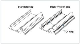
2. On horizontal installs, clips must be installed with the spring part of the clip to the bottom edge. The groove along the rear of the clip indicates the centre line of the Hi-Lite™ 30 tube once installed. Use fixings with head diameter between 7mm (0.3") and 9mm (0.35").
