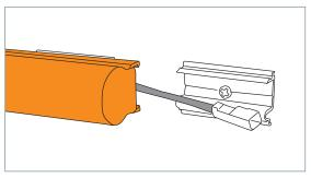
8. Hi-Lite™ 30 tube section clipped in place, with the cable positioned ready to connect to the next section.
