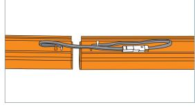
11. Viewed from the rear of the tube, the connection is hidden within the rear channel. When fixing the second section, check carefully that the cables are not trapped and sit freely between the tube and the clips.
