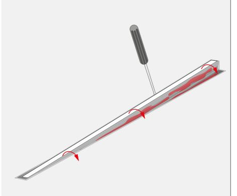
Using e.g. a flat screwdriver, pry up the fixture and remove it from the track.
