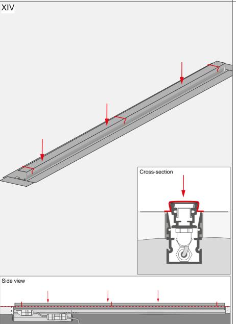
Insert the HR-MAX fixture together with the coupler and cable into the mounting track. The gland of the fixture and the coupler should be in the lower chamber of the HR-MAX-TW profile.
