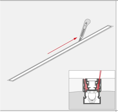
To disassemble the lighting fixture, use a knife to cut the layer of silicone between the wall of the fixture and the mounting track.
