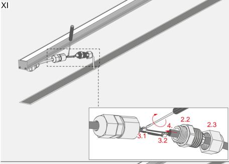
Lead the cable (th)rough items (2.2, 2.3) of the hermetic coupler and attach it to the cable from the fixture, using both items (3.1, 3.2) of the connector.
