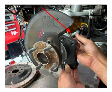
• Note that in the above and below photo the 'flat side' of the bracket faces towards the outside of the car
