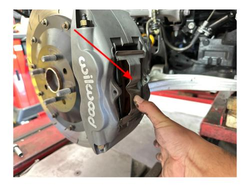
• Slide the bridge bolt back through the caliper with the Allen head towards the outside of the car, and the black, nut facing the inside of the vehicle
