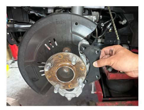
• Install the bracket **to 65-74 lbs/ft torque** using the two factory 17 mm bolts from the back side of the knuckle. It should look like this once it is installed.
