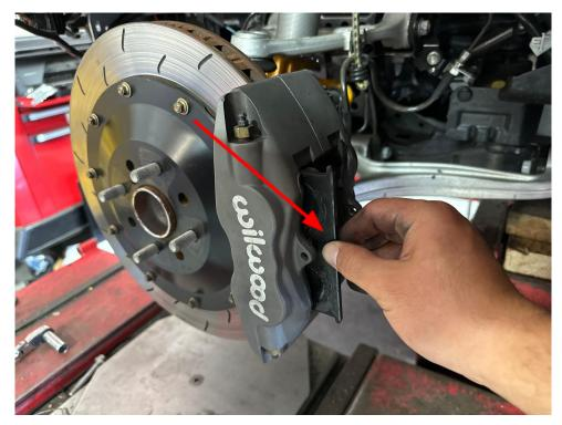
• Next install the caliper brake pad tension clip. Ensure it is lined up correctly, and applying even pressure to all four corners of the inner and outer brake pads, and centered on the caliper itself.
