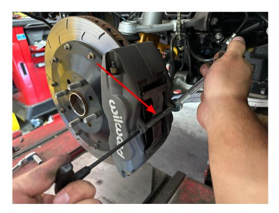
Here's a photo of the tension clip and bridge nut installed completely. Notice that it is centered and contacting all four corners of the brake pads evenly.
