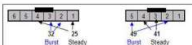
Resistance values as seen in P1 and P2 connectors on the Power Control PCA
