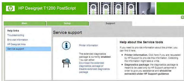
2. If the problem persists and is difficult to debug, try the extended diagnostics package. To enable the extended diagnostics package, click **Enable the extended diagnostics package**. The printer needs to be restarted after enabling or disabling the extended diagnostics package.
