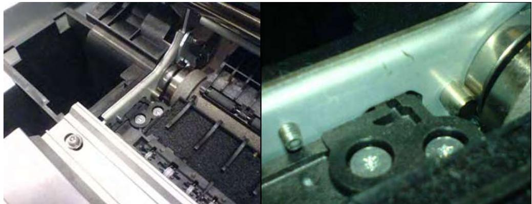
**Problem Description:** Problem with paper advance. This source of error could come from an error in any of the following systems: paper motor, disk encoder, cables or main electronics.
