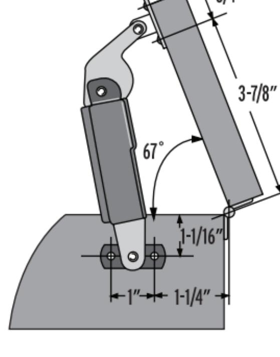
Drill a 3/32" pilot hole using the support as a template.
