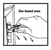
Adjusting the bottom hinge is NOT recommended!
