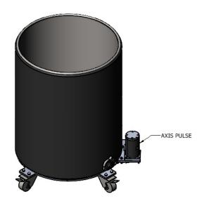
Mount Axis Pulse to Axis Pulse adapter plate using (4) ½-20 x 1 ½" SS button head screw and (4) ½-20 SS self-locking nuts. Use Loctite 270 to prevent loosening. Tighten to a torque value of 6.4 lb-ft.
