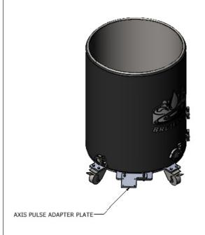
Mount Axis Pulse adapter plate to existing 44 gallon dolly using (4) 5/16-18 x 1 1/4" SS socket head screw and (4) 5/16-18 SS self-locking nuts. Use Loctite 270 to prevent loosening. Tighten to a torque value of 11 lb-ft.
