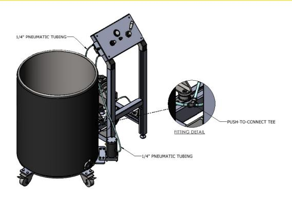
Insert push-to-connect tee by splicing pre-installed pneumatic tubing on pump tand.
