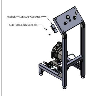
Connect Needle Valve and Bracket to Hash Pump Stand using 5/16" SS self-drilling screws provided. Approximate mounting location to be centered on the stand.
