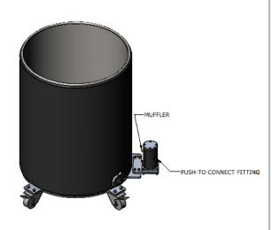
Connect 1/4" NPT exhaust muffler to Axis Pulse.
