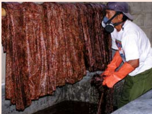
4. The dark mottled background is bleached out but preserved under waxed areas.
