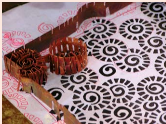
The copper motif elements, stamped across the cloth, must conform to a desired pattern sketch.
