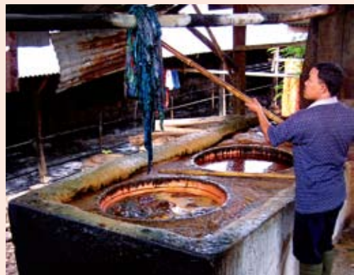
7. Wax is removed by submerging yardage in boiling water.
