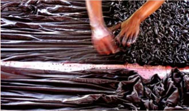
1. Yardage is dyed with base color, then smocked by hand before color effects are created with brushes, squeeze bottles, or sponges.
