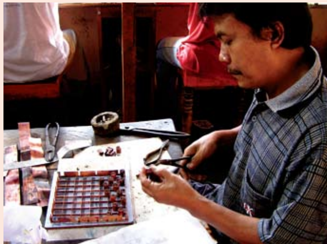
A master cap maker sculpts individual copper motif elements and secures them onto a copper grid.
