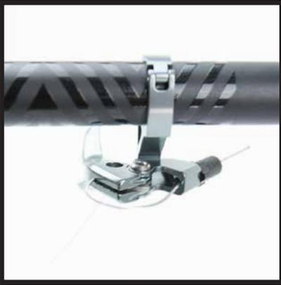
Pull until the cable stops behind the thumb paddle.
