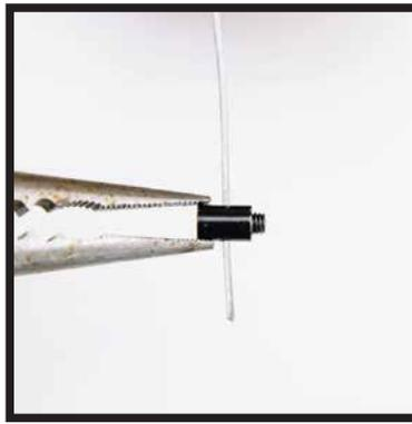
The barrel nut that will be inserted into the lever has a hole for the cable to slide through and is tightened using a 2mm and 3mm allen wrench.
