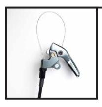
Pull the cable through the lever and hole in the barrel nut until it is taught. The easiest way to do this is to open the lever, thread the cable through the barrel adjuster and create a bit of slack. The cable can now be routed directly into the barrel nut hole.
