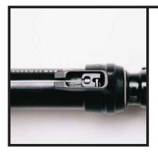
Place the metal cable end into the square shaped insert on the actuator rod.
