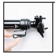
Pop off dust cover at mid-cap. It's easiest to remove from the bottom portion where the cable inserts.
