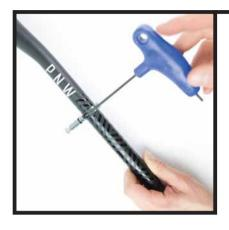
Attach the lever to the lever clamp with a 3mm Allen Wrench.
