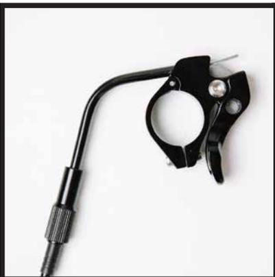
Run the cable through the housing and rotary ferrule to the lever.
