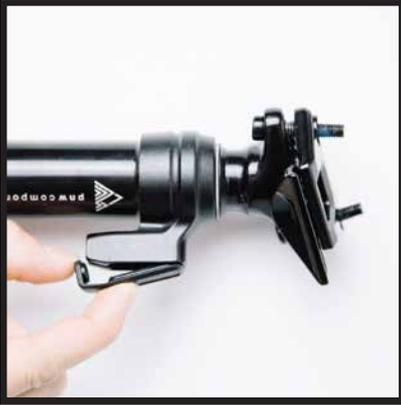
Pop off dust cover at mid-cap. It's easiest to remove from the bottom portion where the cable inserts.
