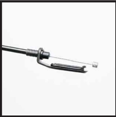
Run the cable through the cable housing and mid-cap dust cover and fix the dust cover to the housing as shown.
