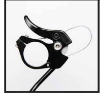
Pull the cable through the lever and hole in the barrel nut until it is tight (easiest to pull with needle nose pliers).
