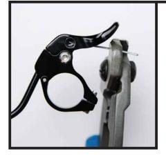
Slide the cable into the guide under the lever (easiest to pull with needle nose pliers)
