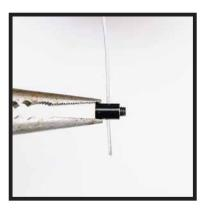
The barrel nut that will be inserted into the lever has a hole for the cable to slide through and is tightened using a 2mm and 3mm allen wrench.
