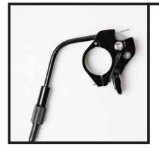
Run the cable through the housing and rotary ferrule to the lever.
