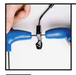
Tighten the bolt with a 2mm allen key on one side and a 3mm on the other side of the barrel nut.
