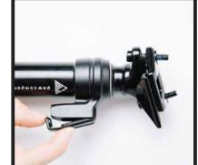
Pop off dust cover at mid-cap. It's easiest to remove from the bottom portion where the cable inserts.
