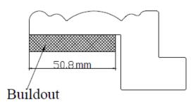
3. For the Deco Frame with buildout, the default is to have a full buildout positioned at the back of the frame. Please see example below of the Camber Deco Frame 50mm:
