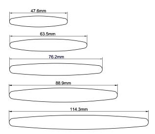
Bermuda louvres are unique and designed like an aircraft wing's, our ABS louvres are strong, rigid and lightweight. Multiple sandings and paint sequences yield an impeccable high-end finish.
