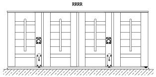
The bolt location for both track system shutters and regular shutters would be the same. The general principle is that the bolt position will avoid the stile which will install the spring-loaded guide at bottom (same stile as the Wheel carrier).
