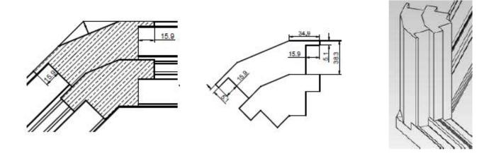
3. For Double Insert Frame 84mm with T-Post , the insert for the Double Insert F Frame 84mm will be cut at the bottom of the posts and there is a 3mm overlap between insert and post. See picture below:
