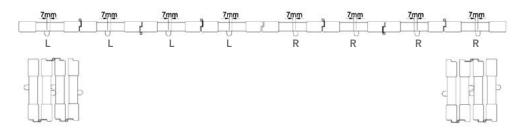
$^{\star}$  For 2 panels (LL/RR) and 4 panels configuration (LLRR), there is no need to offset the tilt rod.
