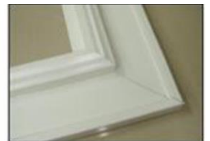
Position the left frame on the Hoffman Key and push down until the frames mitered edges are flush.
