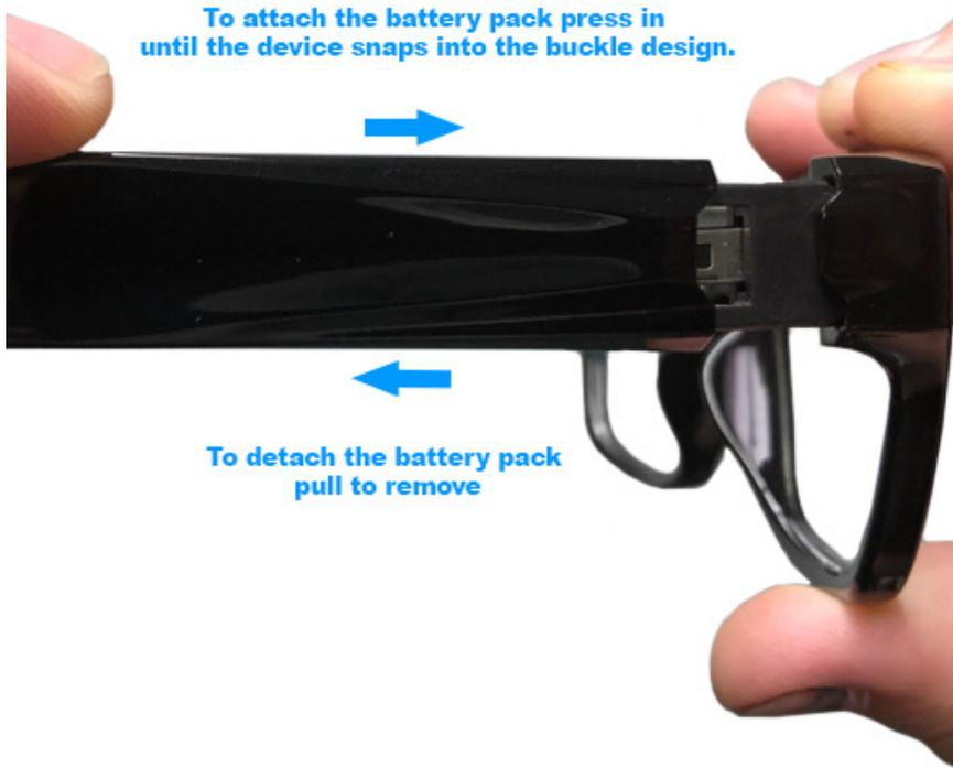
2. To detach the battery pull to remove.
