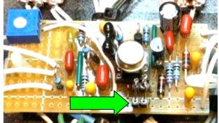
I have the lower one with the cathode(negative) on the left And the upper one with the cathode (stripe) on the right. Flip them in the exact opposite pattern and you will get A more compressed or thinner low mids 80s rawk grind.
