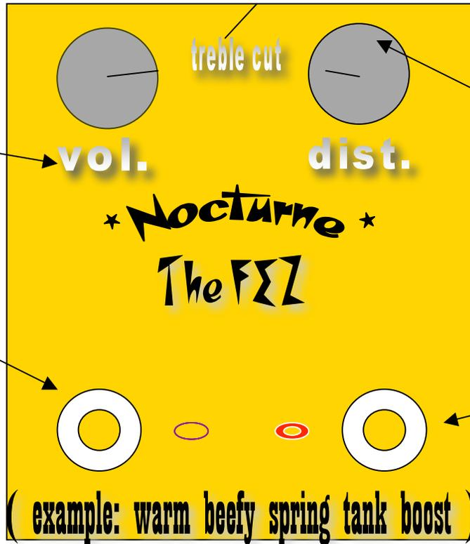
**distortion control,** controls the amount of clipping. Set low for warmer clean boost. Up past 12noon the dirt ramps up with more upper mids bite. Perfect for pushing your amps spring reverb for wetter response with a filthy grind.
