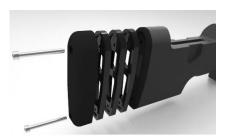
The recoil pad on your PSE rifle stock is fitted to the stock using two M5 screws. To remove the recoil pad and/or a spacer you can use a 4mm allen key. You shouldn't over tighten when re-fitting, just enough so the pad doesn't move. [Please note some stock models may require a 3mm allen key.]
