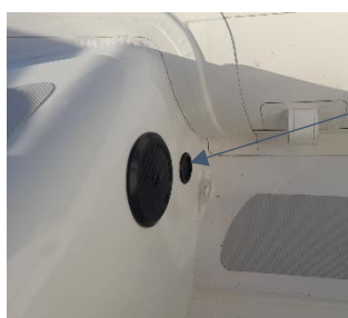
Hull seals for cable runs
