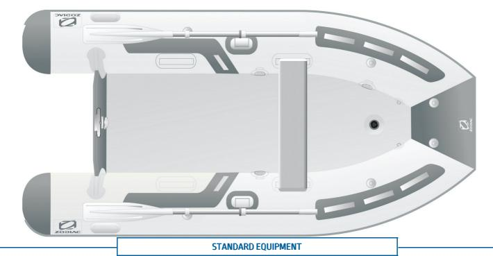
HULL & DECK: 2 Lifting Eyes, 2 Towing Rings, Internally-Operated Bailer. COMFORT: Double Position Auminium Removable Thwart.
