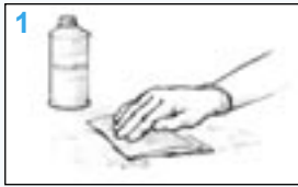
Figure 6 Clean the surface. Use a solvent, if necessary, to remove all contaminants.
