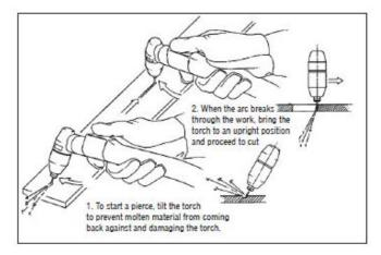
NOTE: Keep moving while cutting. Cut at a steady speed without pausing. Maintain a constant cutting speed so that the arc lag is 10° to 20° behind the travel direction. Use a 5°-15° leading angle in the direction of the cut.
