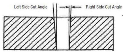
To make a square-edged cut along an inside diameter of a circle, the torch should move counterclockwise around the circle. To keep the square edge along an outside diameter cut, the torch should travel in a clockwise direction.
