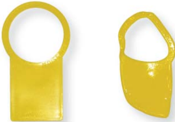
Figure 10 Normal and heat effected test tags
