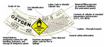
Figure 4 Typical Gas Cylinder Label Information
