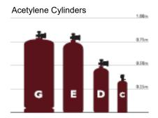
Figure 3 Size Range of Acetylene cylinders Available
