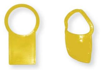
Figure 10 Normal and heat effected test tags
