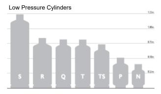
Figure 2 Size Range of low pressure gas cylinders available
