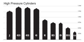
Figure 1: Size range of high pressure gas cylinders available
