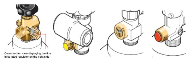
Figure 6 Typical pressure relief devices fitted to cylinder valves. Top Left - Integrated regulator type for 300 atms cylinders, Burst disc type, Fusible plug type, STD pressure relief valve.
