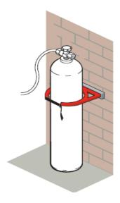
Figure 9 Cylinder secured by wall brackets
