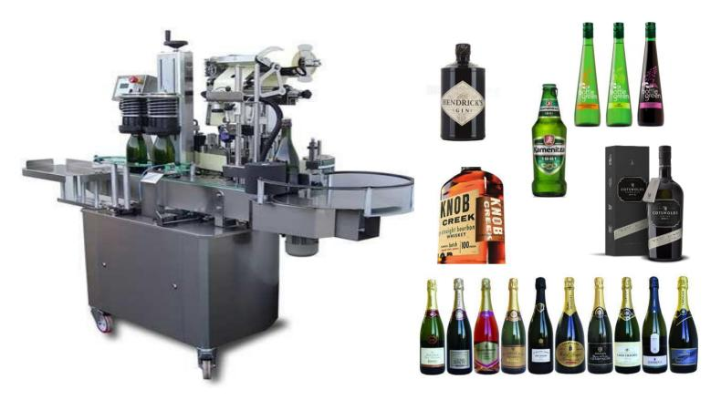
Compact, versatile machines for precise application of multiple labels onto round containers such as 'Champagne' bottles which may be tapered or shaped, Also square bottles, ovals, rectangular and other shapes.
