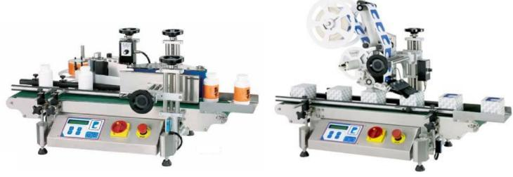
Compact, versatile, and fast, low-cost automatic labellers for either side application onto round containers (LA16a) or top application onto flat –sided items (LA16b).
