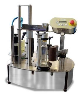
Compact, robust, bench-top machines capable of applying self-adhesive labels from a roll onto a variety of types and sizes of container including cylindrical, tapered, square and shapes.
