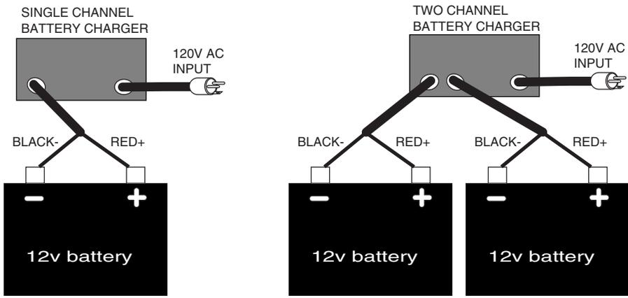
NOTE: If batteries are connected in series for 12/24 - 24V, the series connection wire should be left in place during charging.
