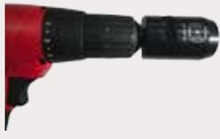
Insert CT-WF38 cable prep tool into a hand drill, and set the drill to medium/high speed. For best results an RPM range of 1,200 to 1,600 is recommended (refer to chart below)
