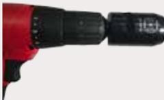
Insert CT-WF14 cable prep tool into a hand drill, and set the drill to medium/high speed. For best results an RPM range of 1,200 to 1,600 is recommended (refer to chart below)
