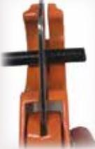
Use CT-CUTTER and insure cable is straight with no bends. For best results, start the blade in a "valley" of the coax. Apply even pressure and rotate the cutter around the cable. This will provide a straight and square cut
