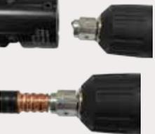
Pull on the drill to remove the center core tool from the rear of the main tool. Place the center core tool over the center conductor and apply pressure, the center core tool will flare out the edges of the outer conductor
