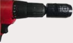
Insert CT-W12 cable prep tool into a hand drill, and set the drill to medium/high speed. For best results an RPM range of 1,200 to 1,600 is recommended (refer to chart below)
