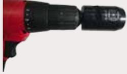
Insert CT-W12 cable prep tool into a hand drill, and set the drill to medium/high speed. For best results an RPM range of 1,200 to 1,600 is recommended (refer to chart below)
