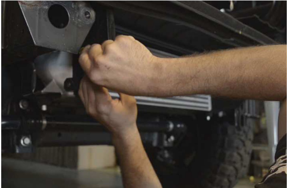
11) There are some hard to find clips that can be popped off with a flat head to remove the rest of the lower air dam
