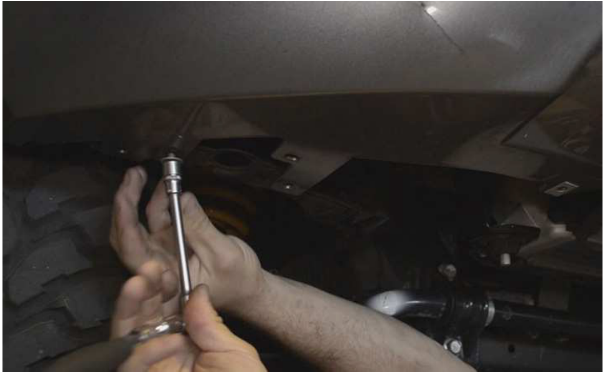
6) Remove the clips holding the inner wheel liner to the bumper.
