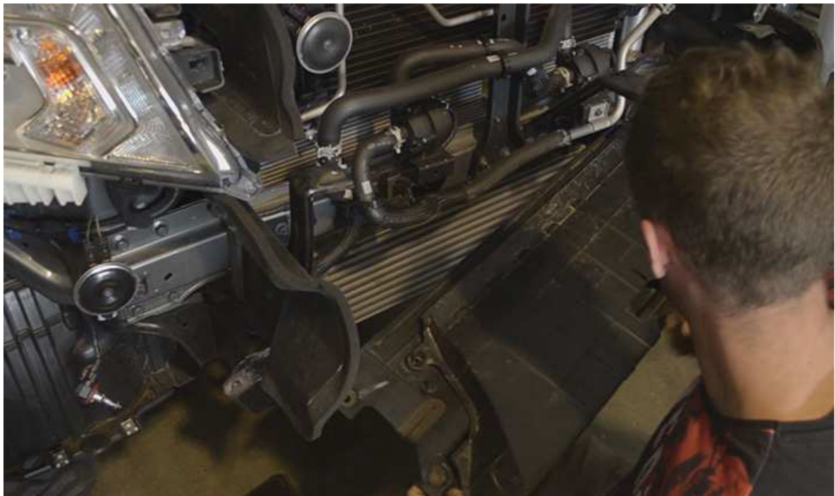
11) There are some hard to find clips that can be popped off with a flat head to remove the rest of the lower air dam
