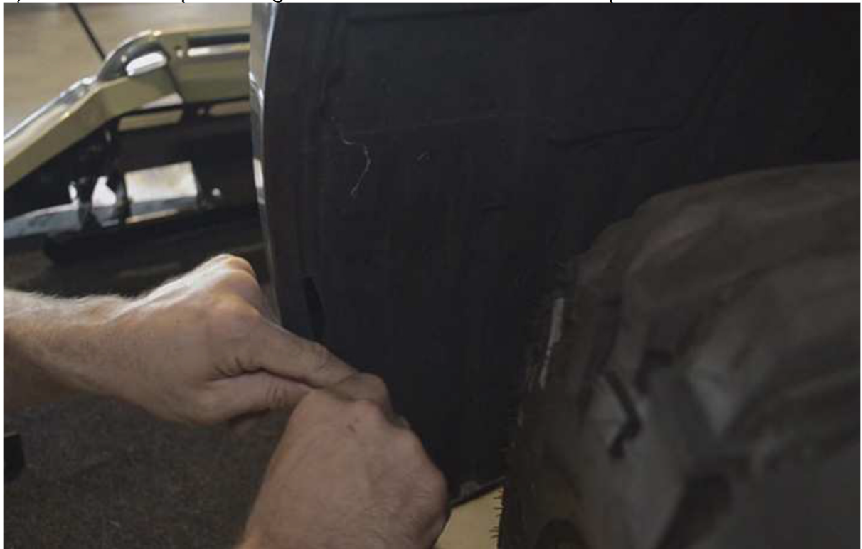
6) Remove the clips holding the inner wheel liner to the bumper.
