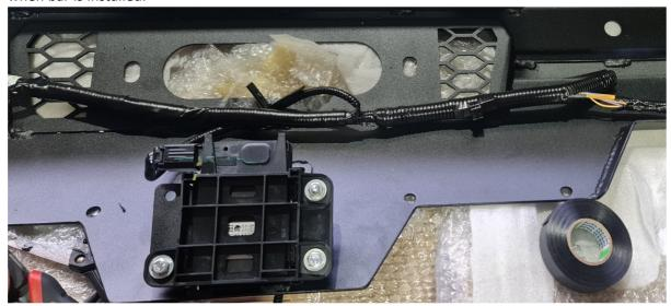
7) The bar reuses factory fog lights, reinstall fog lights install the bar. Passenger side has thinner gauge wires in which if you are wiring up the fog lights you can jumper off this side using the small connector harness, either press clip or solder in. The main fog LED which is larger wattage must be connected via a harness (not supplied) or recommended that you connect those when wiring a led bar (in parallel) the standard arrangement is to connect
