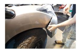
4. Remove the clips holding the top of the grill.
