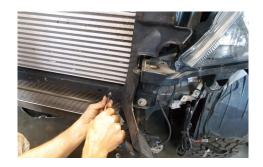
16. Trim the factory air dam as shown, cutting diagonaly up.
