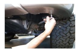
8. While you're down below, remove the factory bash plate, making sure you keep the two rear bolts to use later.
