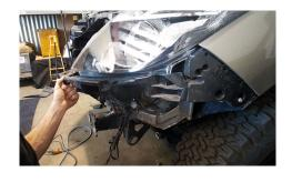
20. Strip the factory fog light wiring ready to solder on the new LED fog lights.
