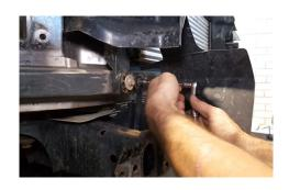
14. Tear away the plastic moulding that is between the chassis rail and the condensor.
