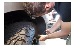
3. Now pull the edges of the bumper away from the car. The clips will pop away and this is completely normal.
