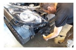
CAUTION: INNER GAURD CUT PARTIALLY EXPOSES AIR INTAKE. SECURE GAURD & TAKE CARE DURING WATER CROSSING. TURN INTAKE UPWARDS OR GET A SNORKEL FOR WATER CROSSINGS
