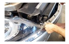
7. Undo the bolts holding the bottom of the bumper to the car.
