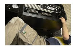
26. Refit the grill with the factory push clips.
