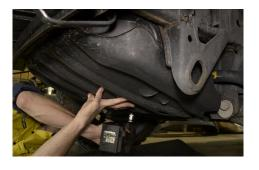
11. Tear away the lower section of the air dam. This can be disposed as it is not needed with the new bullbar.
