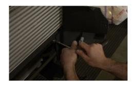
14. With the air dam removed, you can now unscrew and remove the two L brackets. With the L brackets removed, refit the two air dams.
