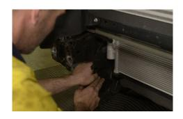
16. Remove the metal brackets underneath the headlights and dispose.
