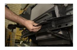
12. Unbolt the crash bar and dispose, this will be replaced by the bullbar mounts.
