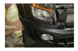
10. Undo the 4 bolts underneath to remove the factory bash plate.
