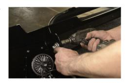
18. Trim the upper air dams down, checking clearance against the mounting bracket and ensure that the sensor on the passenger side air dam is relocated.
