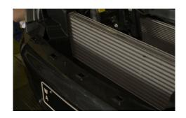
4. Remove the two screw in plastic plugs on the bumper that were covered by the grill.
