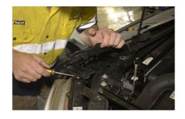
3. With the top 5 push clips removed, the grill can be pulled back and there are 5 clips that can easily be undone where the grill meets the bumper.
