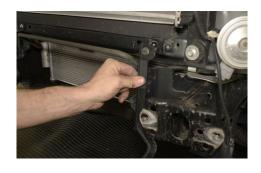
15. Remove the plastic trim down between the chassis and the condenser
