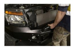
22. The bar should sit with a fingers width gap between the lights and the bar. Once the bar is aligned correctly, tighten all the mounting bolts.
