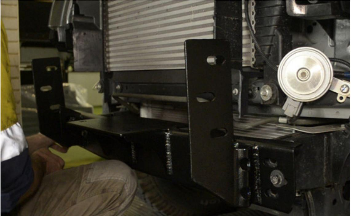
**INSTALL THE SUPPLIED CHASSIS REINFORCEMENT BRACKETS & COMBINED RECOVERY POINT**
