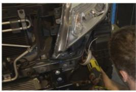
8. Carefully mount the Extreme Series bar it is best to get someone to help you. The bulbar alignment can be difficult. Its best to have bolts loose enough so two persons can hold the bar in place while a 3<sup>rd</sup> tightens the bar. If you are installing by your self alignment can be difficult its suggested you tighten 1 side enough so it can still move under pressure and wedge foam (or similar) between bar and fender to retain gap when lifting the other side into place.
