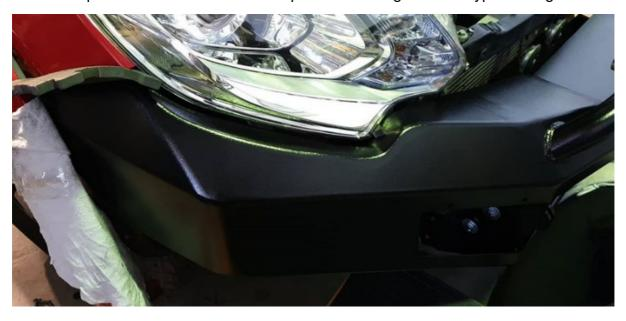
This will create an even gap on both sides, vs trying to align 1 side at a time. We also recommend using same foam under the head lights to maintain the correct gap
