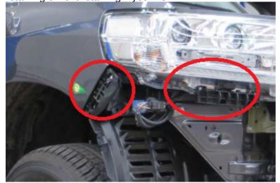
SIDE RETAINER MUST BE REMOVED UNDER HEADLIGHTS YOU CAN PAINT BLACK OR REMOVE ENSURE MAINTAIN GAP IF LEAVING
