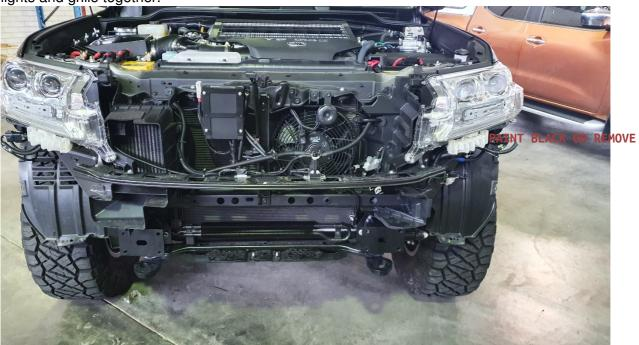
3) Remove grill, front bumper bar, bumper reinforcement and lower bumper support brackets. Also remove bumper retaining clips on side guard, and below headlight as indicated including the plastic side bumper
