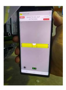
Download Level App Radar Must be max 1.5Degree. 0 Degree level optimal
