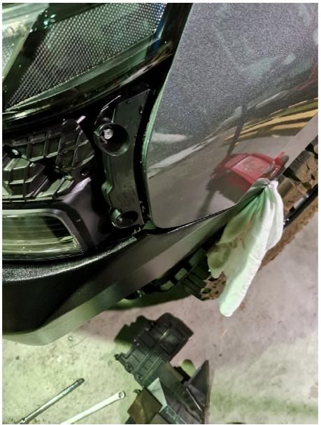
Remove the black bumper retainer shown in this photo held in by 2x 10mm bolt screws.
