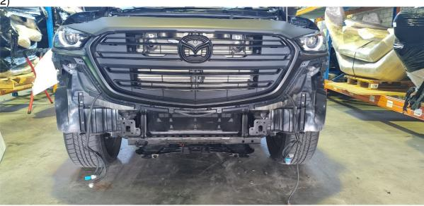
The bullbar comes with chassis reinforcement collars, install these before installing the main winch cradle. The collars go on finger tight.
