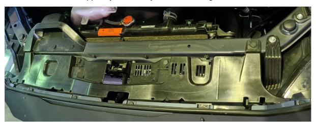
Various clips on the top of the engine bay area, Screw behind the logo, screws under the plastic flap shown in the image. Various bolts under the car. Remove the retainers holding the inner plastic arch to get access to inside and remove the bolts holding plastic bumper to car.
