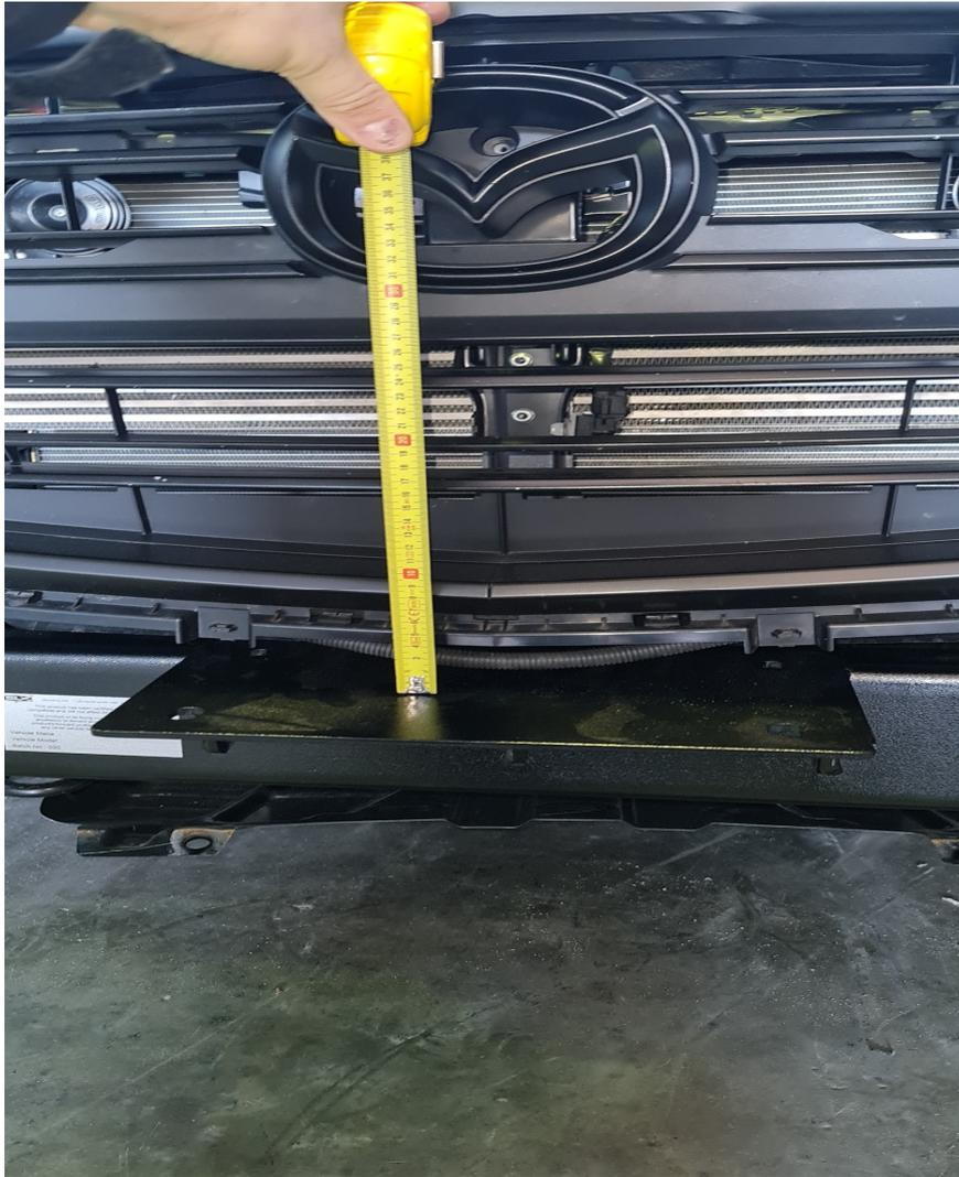
If you are installing a winch you will need to cut the grill to suit your winch height. Install bolts finger loose so you can move bar left to right and back forth(tilt)
