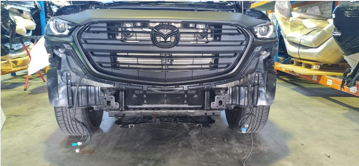
The bullbar comes with chassis reinforcement collars, install these before installing the main winch cradle. The collars go on finger tight.
