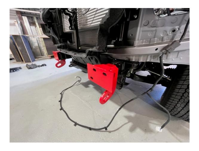
Step 11: Install Bar/Winch Mounting Bracket using 4 supplied bolts (Black) with washers.
