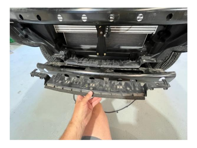
Step 9: Remove 4/14mm Bolts to remove front bumper support and discard. It will not be reinstalled.
