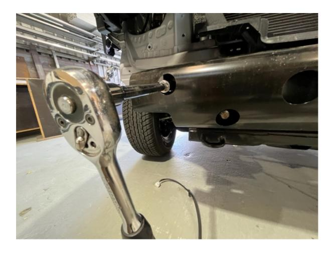
Step 10: Slide 2 Recovery point brackets over end of Chassis and install 100mm Bolts through chase with Nyloc Nuts and washers. Leave loose. Do not tighten till later.
