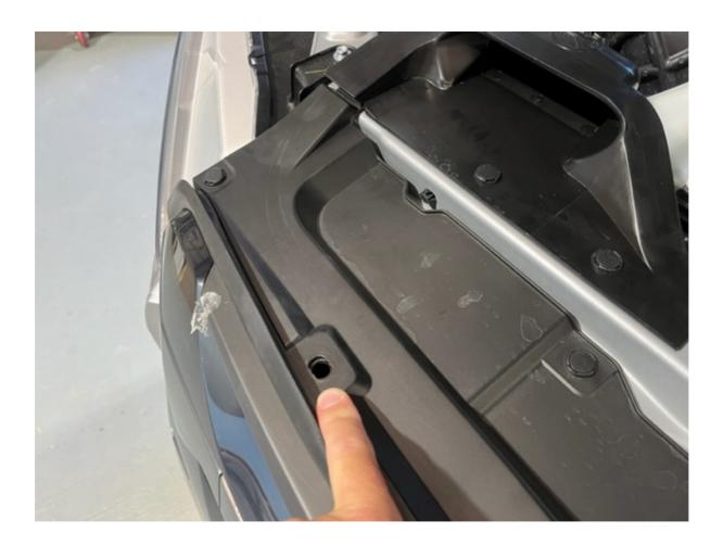
Step 2: Remove retention clip and screw to front of grill and remove top grill section.
