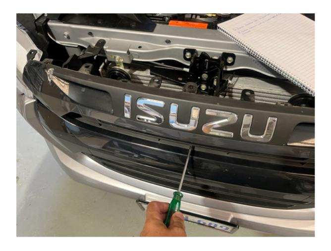
Step 3: Remove retention Clips to top of bumper grill.
