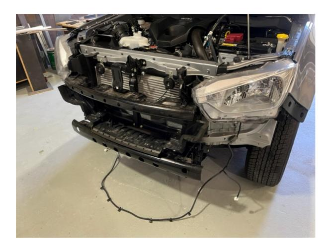
Step 8: Remove/unclip plastic air flow director. If no wince will be added, this part can be reinstalled.
