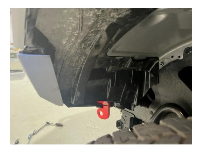
Step 18: Install 2 side lower bash plates with Bolts provided.
