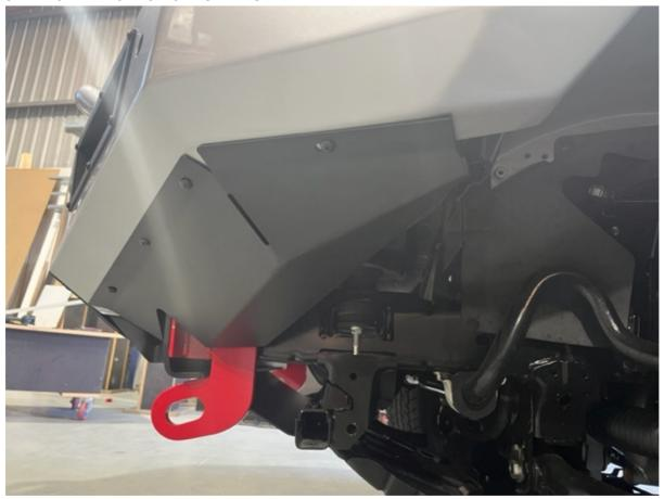
Step 19: Install center baseplate with bolts provided. Reuse 2 bolts from factory to mount bashplate to existing location.
