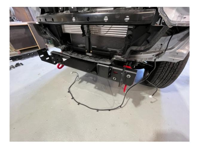
Step 12: Drill a pilot hole then drill a 12mm hole to third bolt location and install supplied M12/35mm bolt with upgraded washers and Nyloc nuts.
